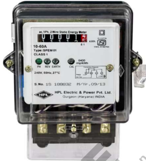
Figure 19. Energy Meter (example of integrating instrument)
