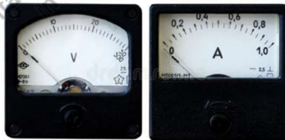
Figure 17. Ammeter-Voltmeter (Example of indicating instrument)
